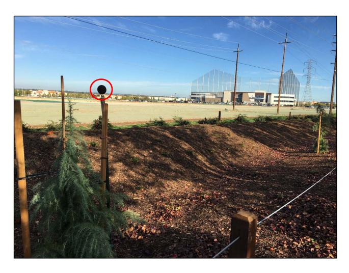
Microphone at end of 5 foot PVC boom attached to tree stake at location indicated.
