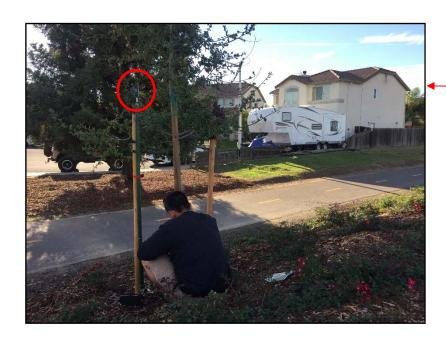
Microphone at end of 5 foot PVC boom – photo shows calibrator attached during setup.
