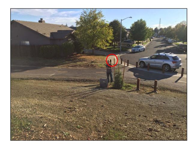
Microphone ultimately placed at end of 5 foot PVC boom attached to tree stake at location indicated.
